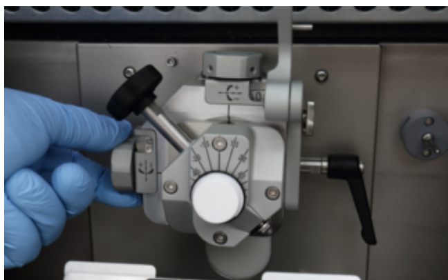
Precise adjustment of face angle.
